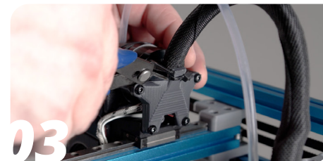
03 Cut more zip ties on the toolhead.
