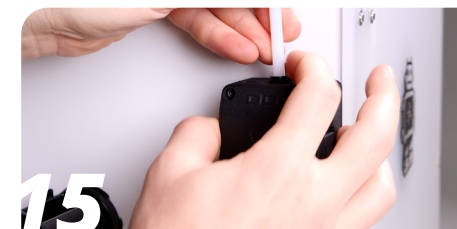
Attach the collet clip and you're done!
