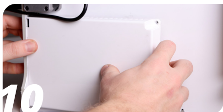
Reinstall the electronics compartment cover.
