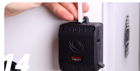
Add the bowden tube to the extruder.
