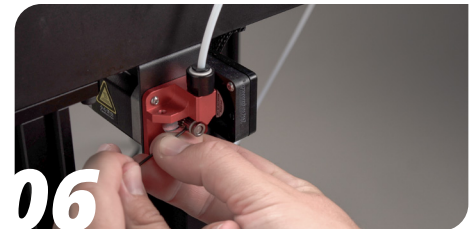
06 Loosen the extruder gear set screw using a 1.5 mm hex key.
