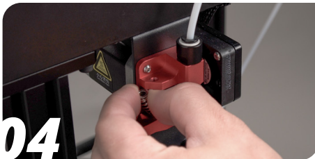
04 Remove the spring.
